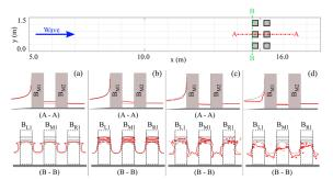
Figure 2 - Comparison of the predicted maximum wave runup on the first row of structures at sections (A-A) and (B-B). The gray and red lines represent the maximum wave runup in the absence and presence of currents, respectively. (a) wave+stronger following current; (b) wave+weaker following current; (c) wave+weaker opposing current; (d) wave+stronger opposing current.
