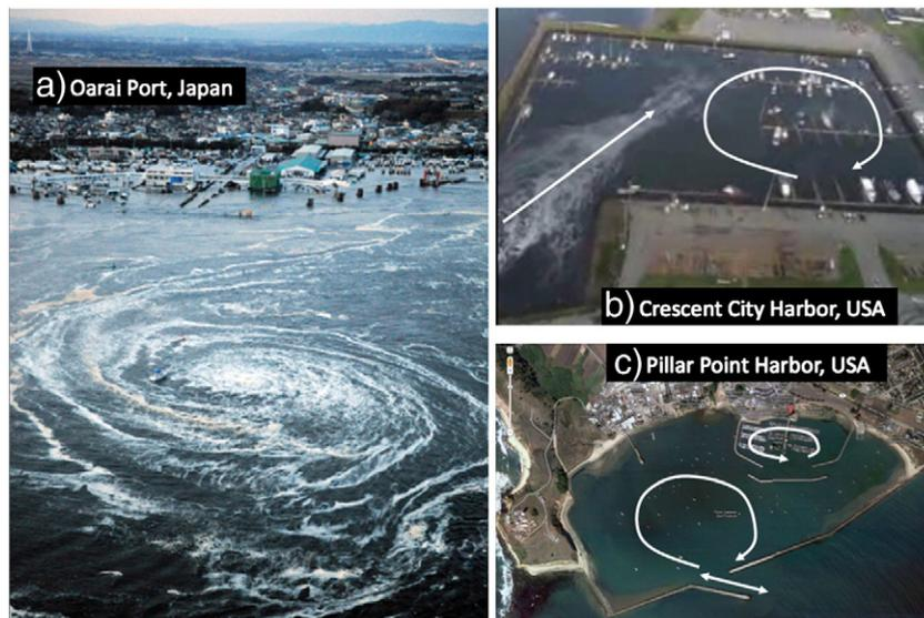
Fig. 1. Selected sites where significant tsunami currents were observed during the Tohoku tsunami. (Left) Port of Oarai and the shallow turbulent coherent structure; (top right) tsunami surge jetting in to Crescent City’s inner harbor; (bottom right) Pillar Point Harbor which experienced counter rotating eddies in the inner and outer basins.
