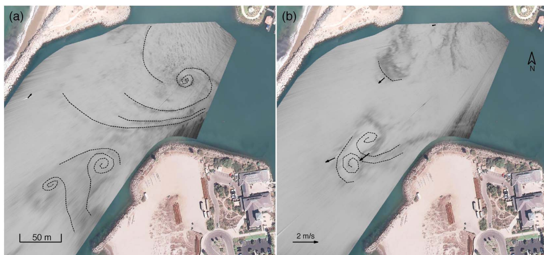
Figure 5. Rectified camera frames captured at (a) 8:29 and (b) 8:43 A.M. local time, overlaid over orthorectified USGS aerial imagery (times are shown in Figure 2 with vertical dashed lines). (a) Transitional jet and TCS forming when flow reversed toward the harbor and (b) two transitional jets expelled from the channel bifurcation corners. Vectors correspond to tracer flow speeds. TCS streamlines and the fronts of transitional jets are approximately shown with dashed curves.
