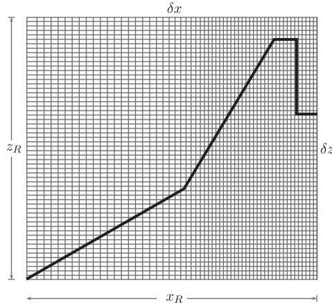
Figure 15. RANS computational mesh for hybrid simulation of BEB sinusoidal wave overtopping.
