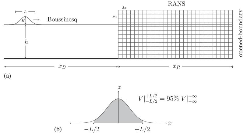
Figure 5. (a) Hybrid simulation setup for solitary wave propagation and (b) solitary wave form centered at the coordinate origin and symmetrical about the  $z$  axis. Gray area occupies 95% of the total water volume in the wave.
