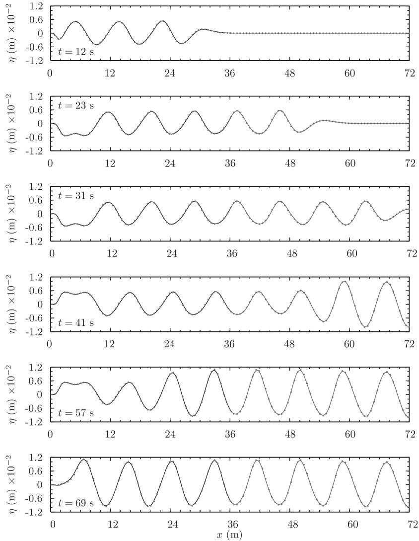
Figure 10. Standing wave ( $\varepsilon=0.02$ ,  $\delta=0.06$ ) motion in a 0.5 m deep channel simulated using the hybrid model.  $0 \leq x \leq 36$  is Boussinesq model,  $36 \leq x \leq 72$  is RANS model, and dots are the full-Boussinesq model.
