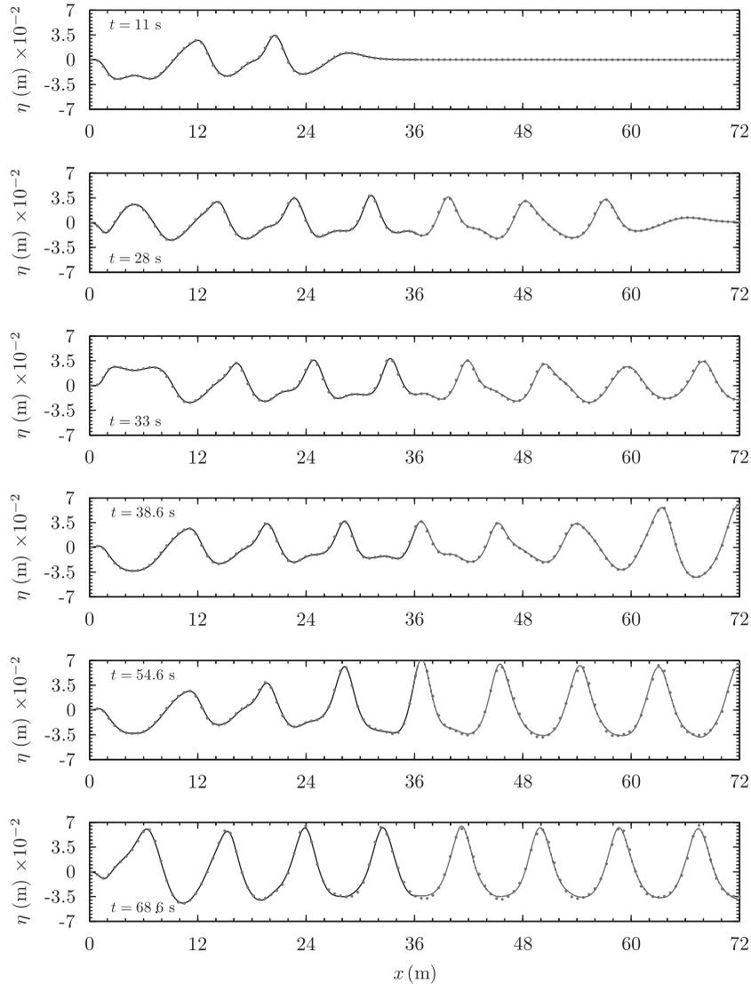
Figure 12. Standing wave ( $\varepsilon=0.1$ ,  $\delta=0.06$ ) propagation in a 0.5 m deep channel simulated using the hybrid model.  $0 \leq x \leq 36$  is Boussinesq model,  $36 \leq x \leq 72$  is RANS model, and dots are the full-Boussinesq model.
