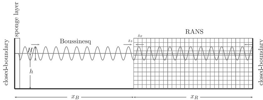
Figure 9. Hybrid model setup for standing wave simulation.
