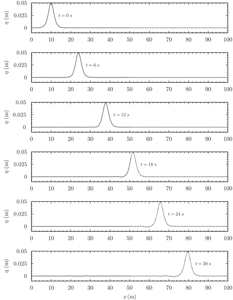
Figure 6. Solitary wave ( $\varepsilon = 0.1$ ,  $\delta = 0.075$ ) propagation in a 0.5 m deep channel simulated using the hybrid wave model.  $0 \leq x \leq 50$  is Boussinesq model,  $50 \leq x \leq 100$  is RANS model, and dots are the full-Boussinesq model.
