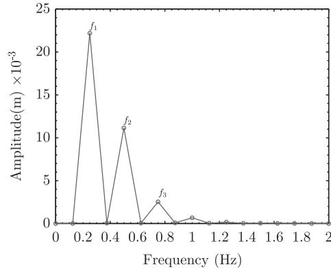
Figure 13. Amplitude spectrum of the free surface elevation time series of the  $\varepsilon=0.1$  standing wave simulation. The time series is recorded at  $x=38.0$  m and before the reflected wave reaches this location.
