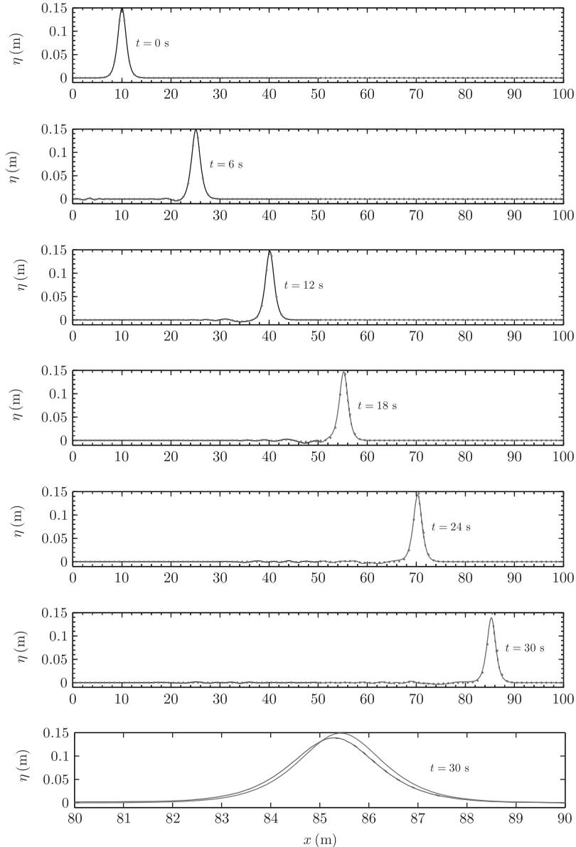
Figure 7. Solitary wave ( $\epsilon=0.3$ ,  $\delta=0.12$ ) propagation in a 0.5 m deep channel simulated using the hybrid wave model.  $0 \leq x \leq 50$  is Boussinesq model,  $50 \leq x \leq 100$  is RANS model, and dots are the full-Boussinesq model.
