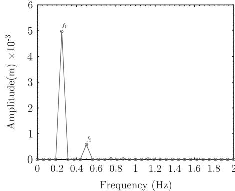
Figure 11. Amplitude spectrum of the free surface elevation time series of the  $\varepsilon=0.02$  standing wave simulation. The time series is recorded at  $x=38.0$  m before the reflected wave reaches this location.
